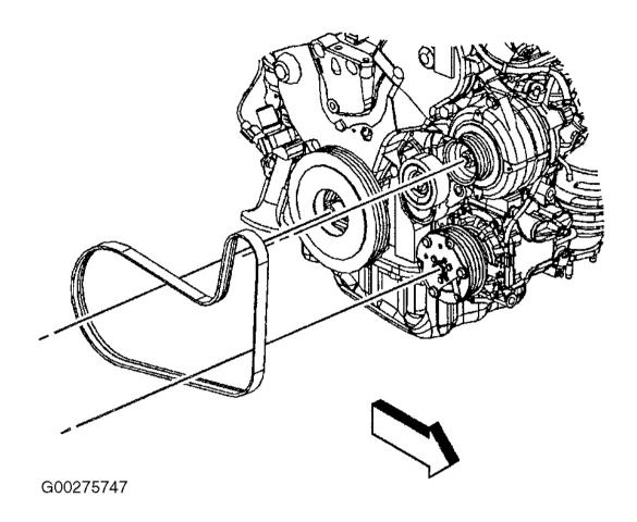
Fig. 2: Identifying Belt Routing (3.5L) Courtesy of GENERAL MOTORS CORP.
