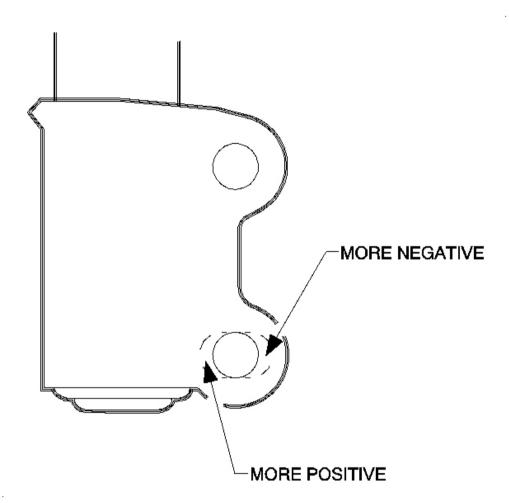
Fig. 2: Strut & Knuckle Courtesy of GENERAL MOTORS CORP.
