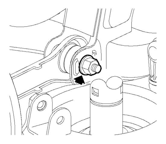
Fig. 7: Toe Link-To-Frame Fastener Courtesy of GENERAL MOTORS CORP.
