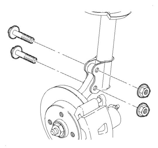
Fig. 1: Strut, Knuckle Nuts & Bolts
