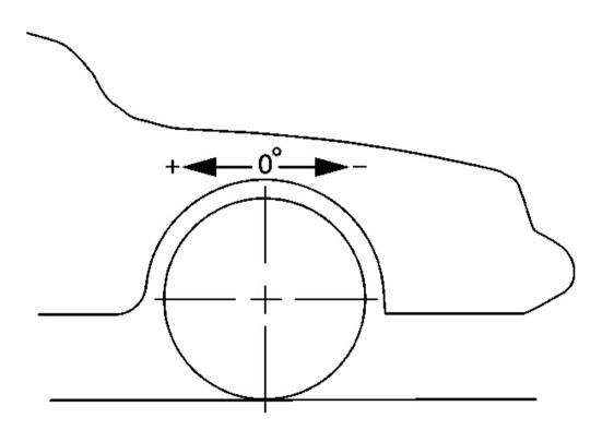
Fig. 8: Illustrating Caster Angle Courtesy of GENERAL MOTORS CORP.
