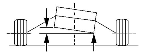
Fig. 12: Identifying Torque Steer Courtesy of GENERAL MOTORS CORP.
