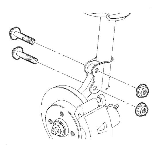
Fig. 3: Strut, Knuckle Nuts & Bolts
