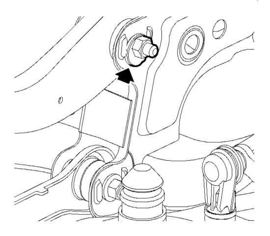
Fig. 6: Upper Control Arm-To-Frame Fastener Courtesy of GENERAL MOTORS CORP.
