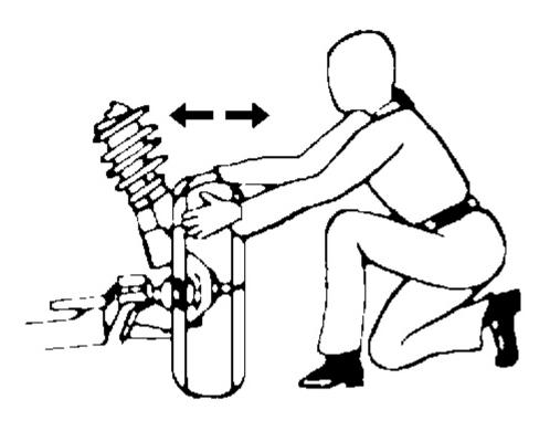
Fig. 4: Adjusting The Camber Specifications By Moving The Top Of Wheel In Or Out Courtesy of GENERAL MOTORS CORP.
